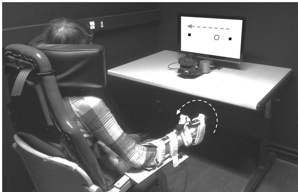
Fig. 1 Test set-up. Participants placed their right forearm into an orthosis while seated in front of a computer screen showing two fixed square targets and a round cursor. Wrist flexion and extension movements moved the cursor towards the left and right of the screen, respectively. In the CONTROL condition, participants were asked to move the cursor as fast and accurate as possible from the right (start-
